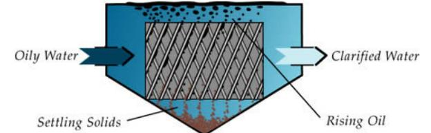
reaches the top of the media plate the droplet pulls away from the plate and rises to the water surface. To some degree, the solids replicate this process in reverse (settling).
